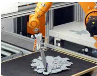
Robotic loading offers maximum flexibility. Blanks can be loaded from a bulk material box or from stacks.
