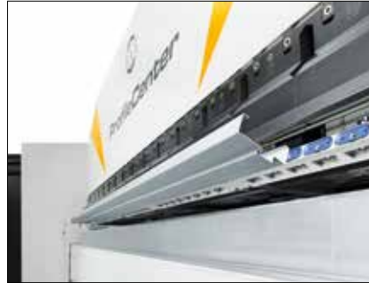
Complex part geometries can be bent due to the large free space around the tools.
