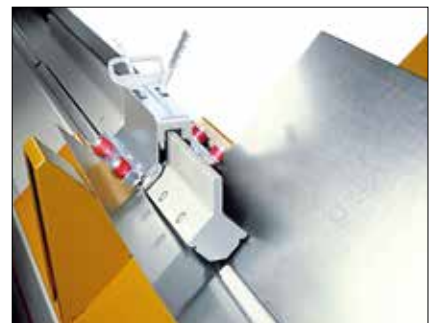
Autopilot and reinforced seaming bar on the RAS 20.12 DuctZipper.
