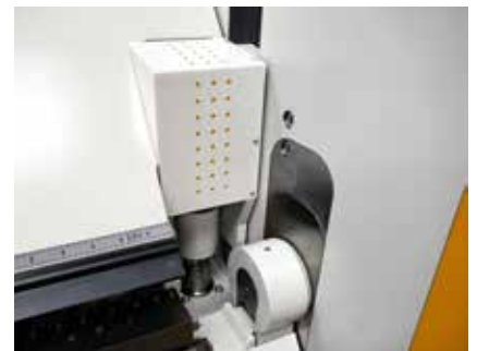
The PowerBooster clamps the blanks with 120 tons of pressure to guarantee straight bends.
