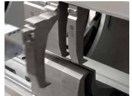
The automatic tool setup allows for quick change-over between parts and the production of small batch sizes.
