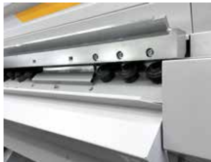
Easily accessible forming rolls for cleaning and maintenance.
