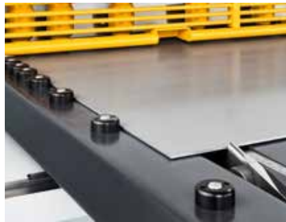
Front stops (available also with a precision scale) allow an accurate part positioning.
