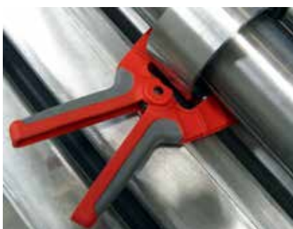
Stiffening pliers reduce shaft deflection for consistent radii.
