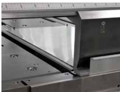
During the folding sequence the sheet rests on the machine table. No need to lift the part.
