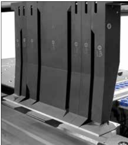
Upper beam tools as tall as 400 mm
