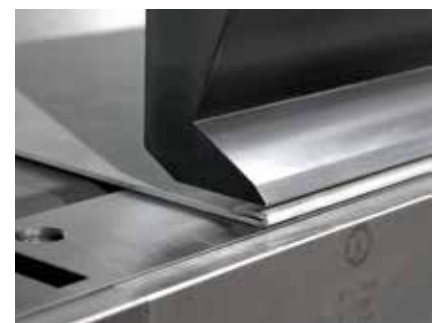
The PowerBoosters offer impressive performance when hems need to be closed.
