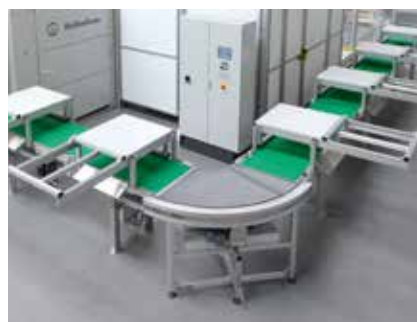
Dedicated unloading of the finished parts depending on floor space conditions, material flow, and sensitivity of the parts.
