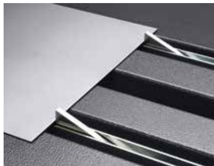
Precise blank positioning by solid stop fingers.
