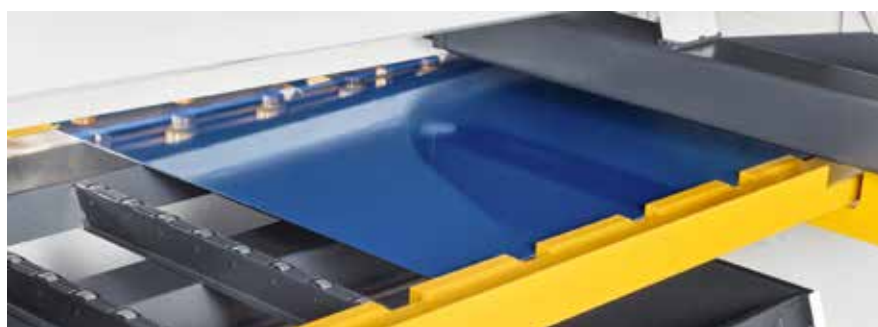
The sheet support system guides even thin materials exactly to the CNC backstop.
