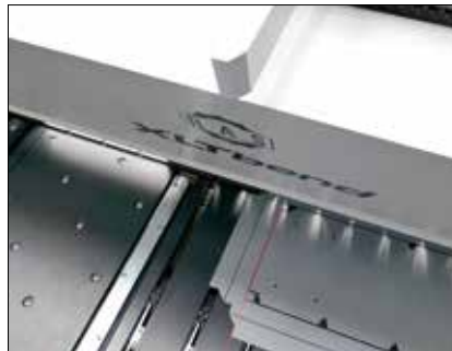
The laser beam of the Virtual Navigator (ViN) shows the exact part loading position.
