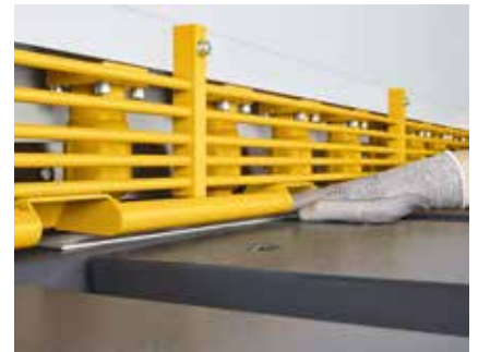
Deep finger pockets for best material utilization.
