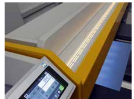
Convenient blank alignment with the LED cutting line illumination.
