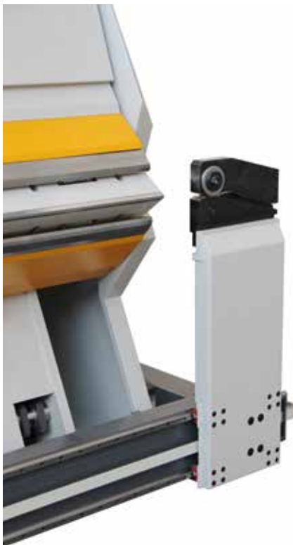
CutModule for trimming wide blanks. Automatic sequence: cutting and bending.
