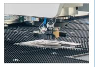
Index equipment and also stripper height adjustment
