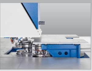
The Multipunch changes tools in 3-5 seconds. Revotools within the same cartridge are changed in less than 3 seconds.
