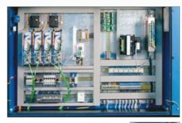
**Electrical cabinet** Open and easily surveyed panel includes digital control, cooling fan, transformers and control.
