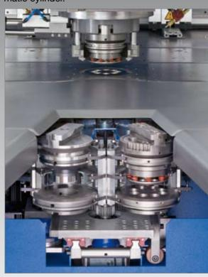
8 station tool carrousel with cassettes that hold punch, die and stripper or Revotool head with
