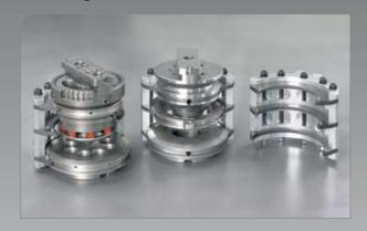
Quick change tool cassettes hold the punch, die and stripper and are set off-line so as not to limit machine run time.
