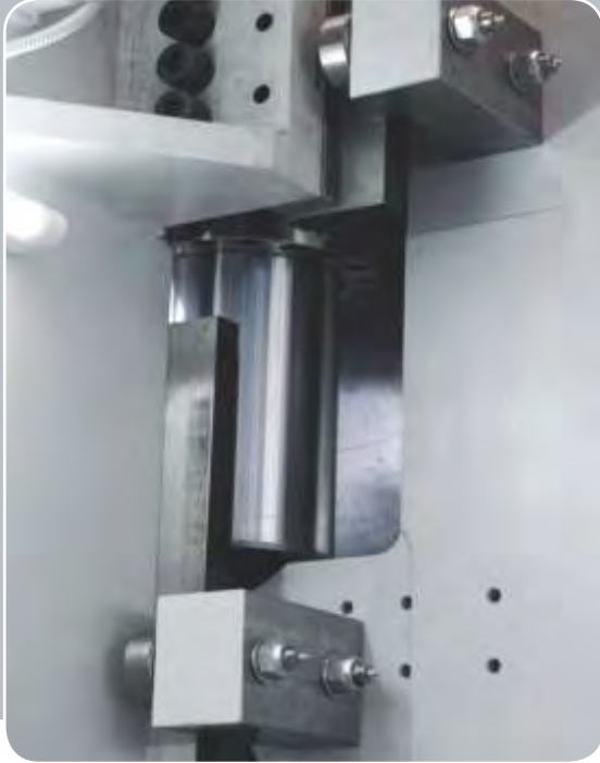
Upper and lower double roller bearing for accurate, rigid and fast beam movement.
