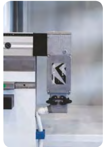
CNC controlled anti deflection system (crowning)
