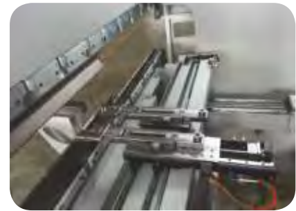
Five (5) axes Back Gauge, including Delta-X, function
