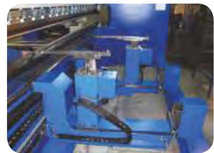
Six (6) axes Back Gauge, X1-X2-R1-R2-Z1-Z2
