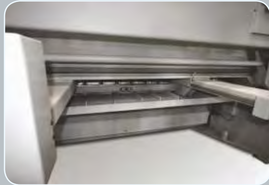
Position 1: Supports the sheet on the back gauge (in the full cutting length). It is not possible the sheet stretch.
