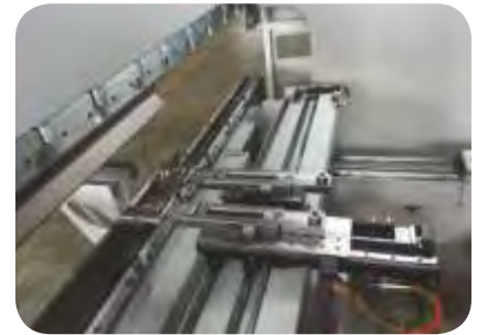
Five (5) axes Back Gauge X-X'-R-Z1-Z2, including Delta-X, function
