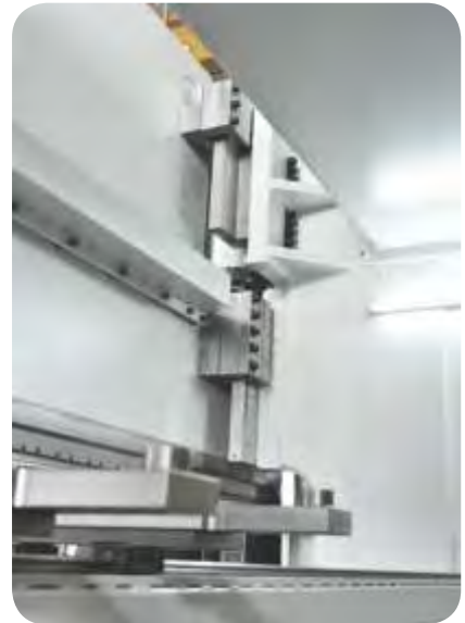
Guiding with Heavy Duty bronze sliders, for a safe and accurate movement of the tool holder
