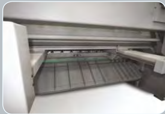
Position 3: Goes down even more, taking a 45° position, guiding the sheet outside the working area of the shear.
