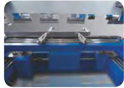
Four (4) axes Back Gauge, X-R-Z1-Z2
