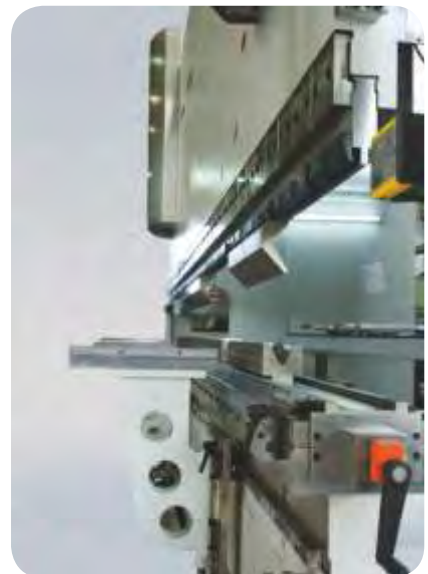
Heavy Duty clamping system (up to 350t/m)
