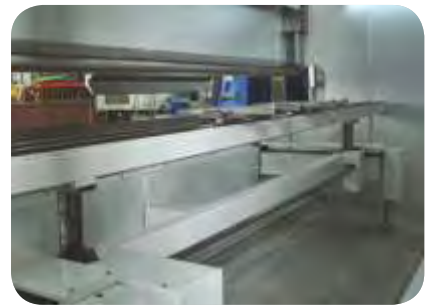
Heavy Duty, two (2) axes, Back Gauge, X-R
