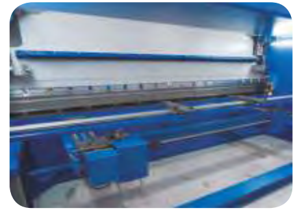
Two (2) axes Back Gauge, X-R
