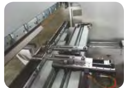
Five (5) axes Back Gauge, X-X'-R-Z1-Z2
