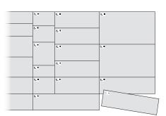
With PROCUT (roller shears with step-cut) and nulT as options, the system calculates how the sheet is to be cut for optimal material utilization without waste. You can also get your cut materials of varying lengths, provided with labels.
