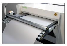
With the STRAIGHT extension, the material is fed smoothly, and the integrated straightening (optional) results in completely flat strips without stop marks. With straightened strips, you facilitate the feeding of your folder and secure the quality of your trims and panels.
