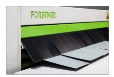
Used in combination with nuIT this machine becomes a marvel of efficiency and precision. Your finished cut pieces are ejected at an impressive speed, up to 25 metres per minute, ready for the next precision step in production.
