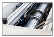
With the unique system for automatic setting of the position of the slitting knives and blade gap, you will get perfect strips in a minimum of time.
