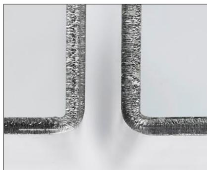
The radius differences are clearly seen in the illustrations above. With a fixed bending centre (left) the radius is uneven and the material is unevenly distributed. With an adjustable bending centre (right) the radius is even and there is less stress on the material.
