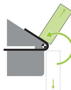
With adjustable bending centre the folding beam follows the radius beam perfectly. The material is bent with an even radius and the risk of cracking and damage on painted surfaces is minimal.
