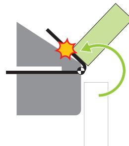
With fixed bending centre there is considerable angle error and a clear risk that the folding beam rail and radius rail "collide" leading to a great deal of wear on the machine or breakdown.
