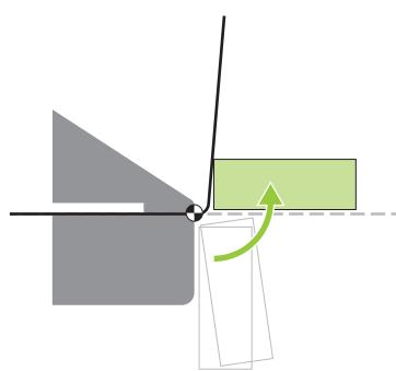
With fixed bending centre, thin material and adjusted folding beam. Good flexibility for angles and limited stress on machine and material.
