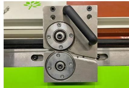
With a simple **rotary shear** attachment along the bend line, you can easily cut off blanks or folded profiles. (Only F41.)
