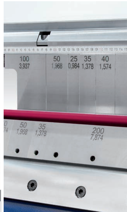
Segmented tools provide flexibility for a variety of geometries.
