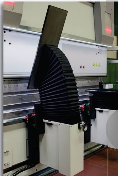
CNC controlled support arms to assist the operator to prevent contrabends
