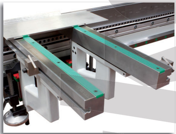
Adjustable support arms to adapt different die heights
