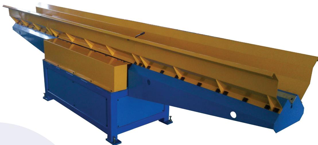
The machine was specially designed for profiling the male and female seam on each side of a rectangular air duct box, as well as to close them. This machine is very effective, productive and economic; furthermore you save manpower as well as the purchase of additional machines.
