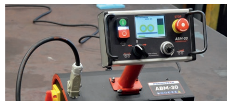
Control panel indicates current work mode and gives safety and diagnostic information
