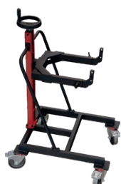
WOZ-0690-20-00-00-0 Screw type transportation and storage trolley with stepless height adjustment
