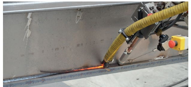
Promotech automatic mechanical-electro joint tracking ensure proper and repeatable welding by means of easy slug removal process.
