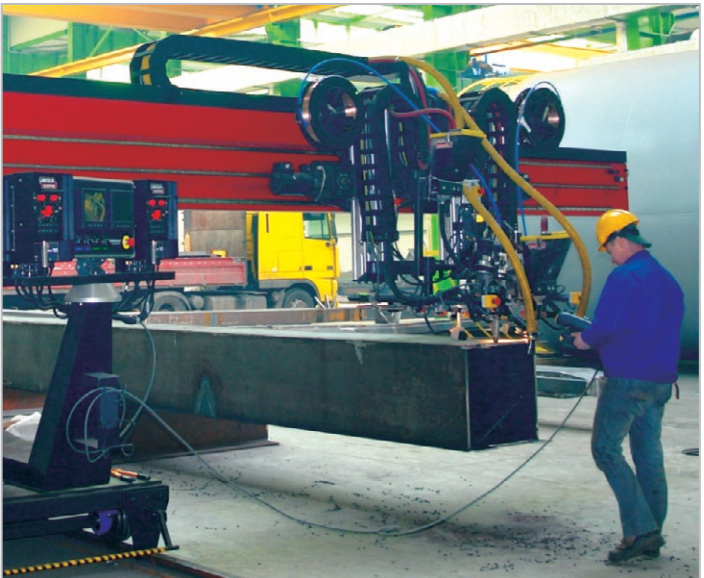
Sample view of C&B operating panel and integrated MIG-MAG welding equipment from (ESAB and LORCH)
