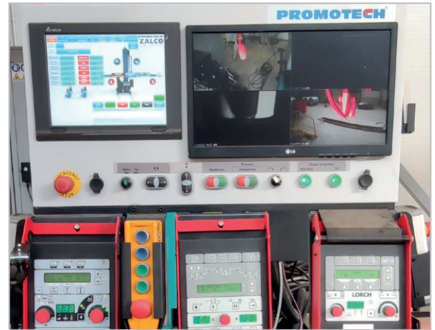
Sample view of C&B operating panel and integrated MIG-MAG welding equipment from (ESAB and LORCH)
