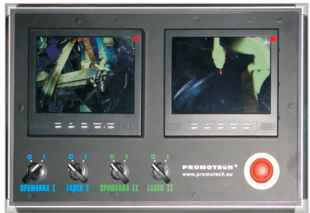
Optional equipment include: camera system for GMAW/SAW, automatic joint tracking system, flux handling equipment, fume extraction, welding rotators, positioners and turntables.
