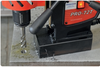
Tapping through holes up to M20
