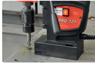
Tapping blind holes up to M20
