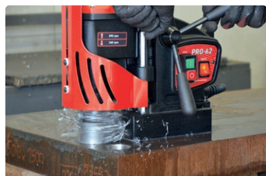
Milling capacity up to 65 mm (2-9/16")
