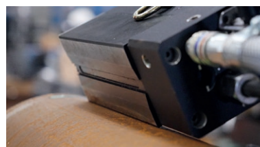
V-shaped prismatic mag base for pipe drilling.
