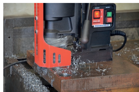
Milling capacity up to 55 mm (2.17") Depth of cut up to 75 mm (3")
