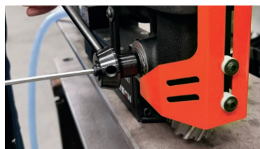
Feed handle can be fixed from either side
