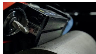
V-shaped prismatic mag base for pipe drilling
