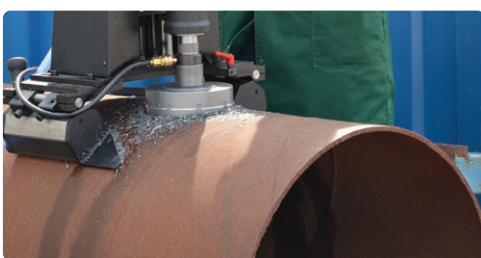
PRO-200A ATEX can be fixed to pipes of min. 950mm (37.4") diameters
