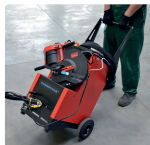
Portable hydraulic power pack with shelf for puncher transport.
