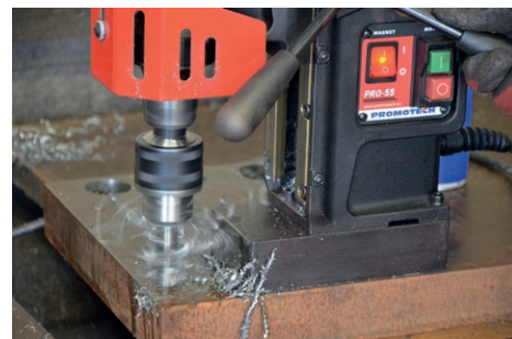
Drilling capacity up to 16 mm (0.63")
