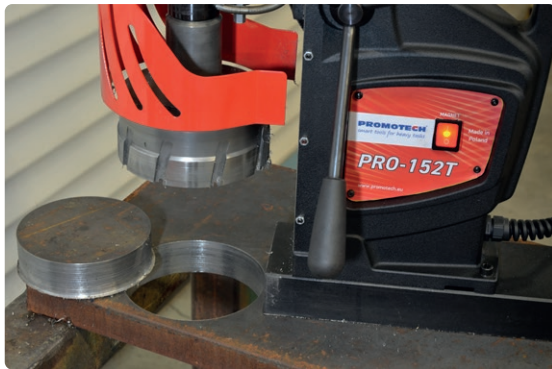
Milling capacity up to 150 mm (5-7/8")
