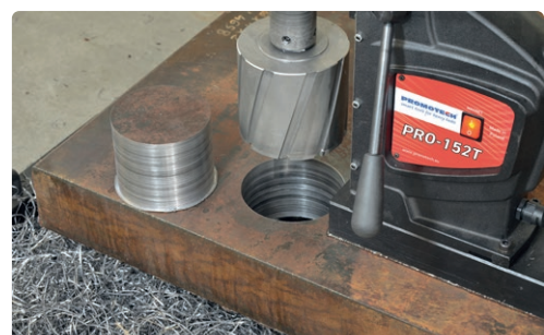
Max depth of cut up to 100 mm (4")
