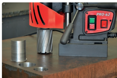
Max depth of cut up to 75 mm (3")
