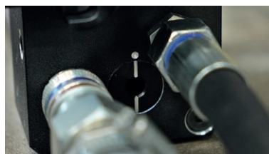
Clamping level indicator for safety and security
