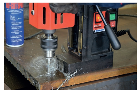
Drilling capacity up to 16 mm (0.63")
