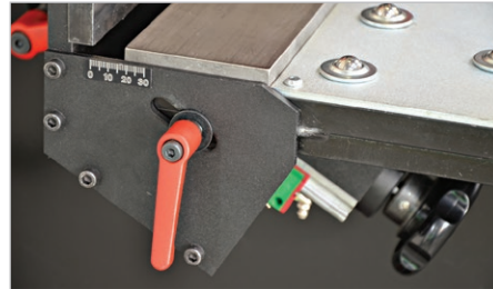
Simple setting of bevel width
