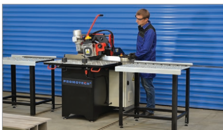
Auxiliary tables to accommodate long workpieces
