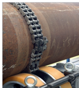
Adjustable chain (Ø 200-1000 mm) ensures positive axial rotation
