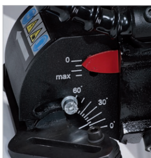
Continuous angle adjustment from 0 to 60 degrees.
