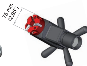
Minimum distance between tubes is 75 mm (2.95")
