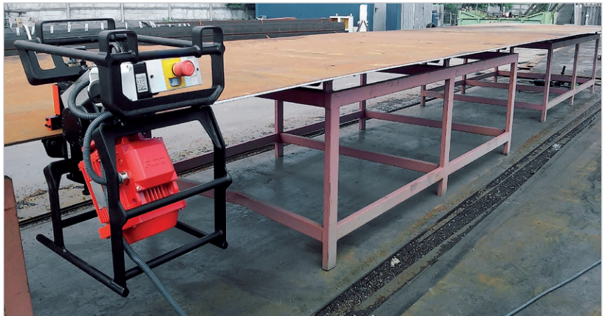
ABM-14 runs along a plate automatically
