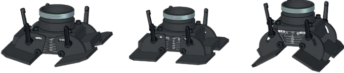
Attachment for removal of welded joints from longitudinal and circumferential surfaces (min. OD 200 mm, min. ID 400 mm) with angle adjustment from -10 to +30 degrees tanged to the cylindrical surface.
