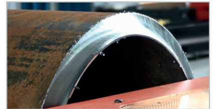
J-groove pipe end preparation (R6 or R8)
