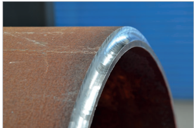
J-groove R8 pipe end preparation
