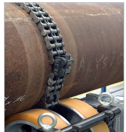
The chain ensures positive axial rotation. Chain length can be adjusted to fit pipe diameters ranging from 200 to 1016 mm
